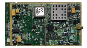
DSP based OEM Radio Modem with Built-in wireless link Monitoring and Management Tools:
