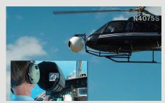
Airborne surveying applications use EMCORE's DSP-3100 to provide the stabilisation necessary to produce clear images.
