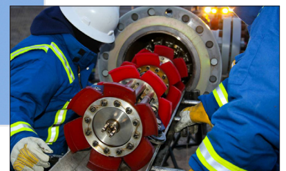
Pipelines deliver massive amounts of crude daily and ensuring safe operation is key. The EMCORE DSP-1760, coupled to additional sensors, provides these inspection robots with extremely accurate angular data.
