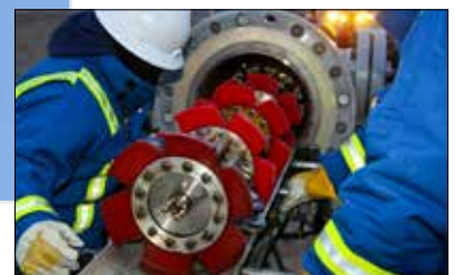
Pipelines deliver massive amounts of crude daily and ensuring safe operation is key. The KVH DSP-1760, coupled to additional sensors, provides these inspection robots with extremely accurate angular data.
